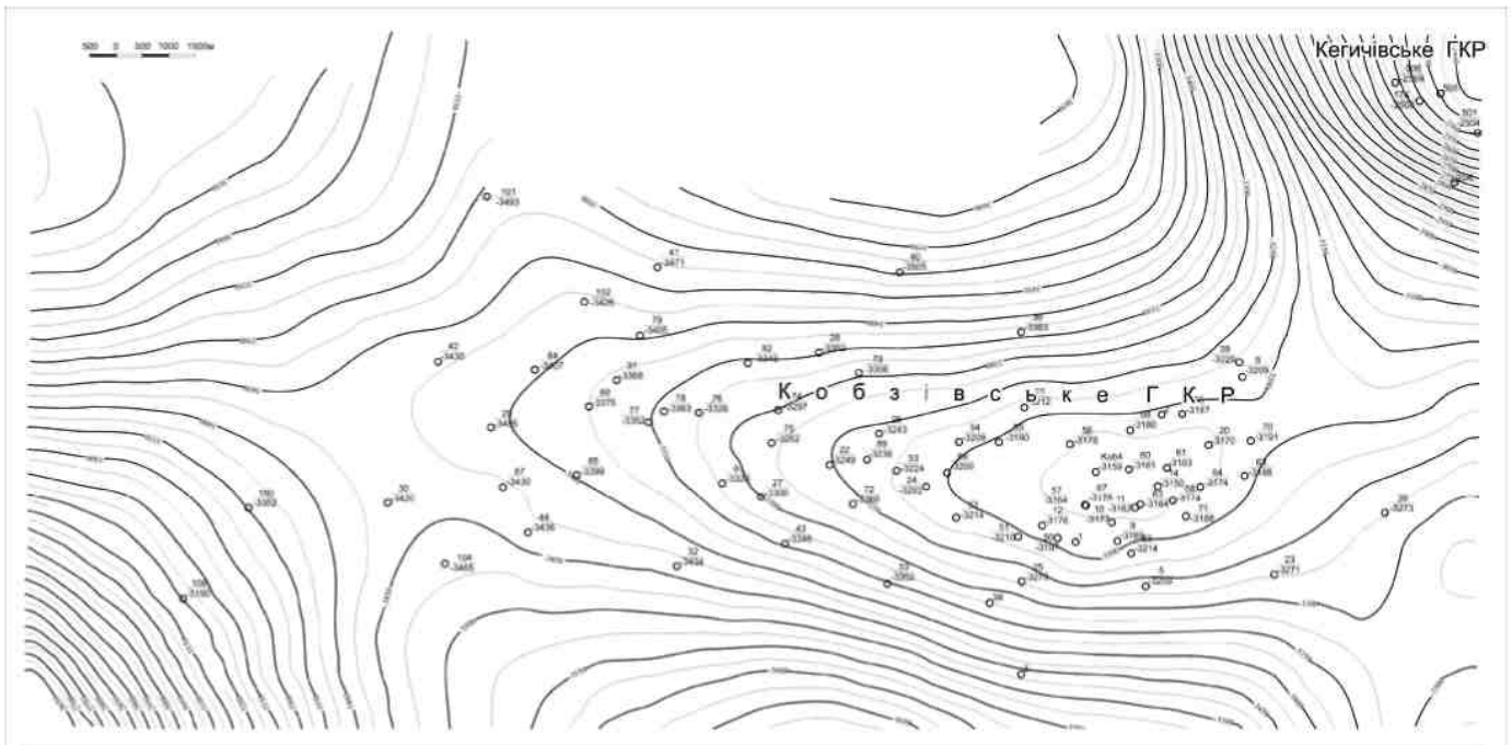
Fig. 1. Kobzivka GCM. Seismic structural map by the reflecting horizon of IV G2
