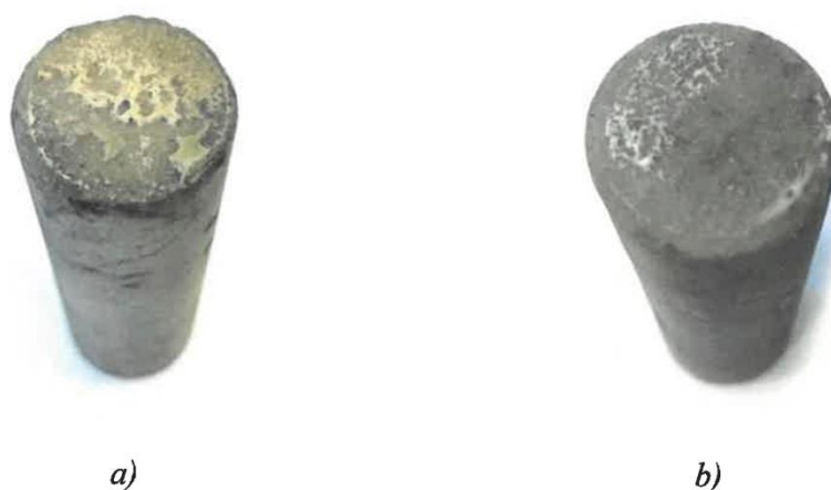
Fig. 4 – Core samples after mud pumping and measuring of final permeability: a) Biocar-TF; b) Biocar-TF + 1% Alevron
